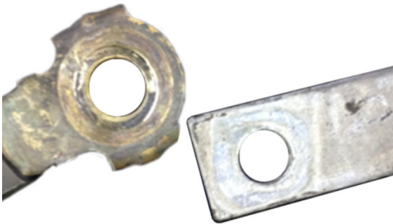
Fig. 1: Ground connection prior to cleaning: Poor connection
