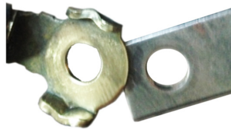
Fig. 2: Ground connection following cleaning: Good connection
