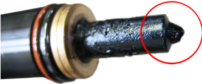
Fig. 3: Unit-injector element coked
